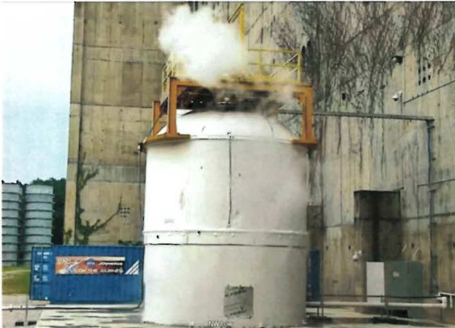
Integrated test article chilled with LN 2
