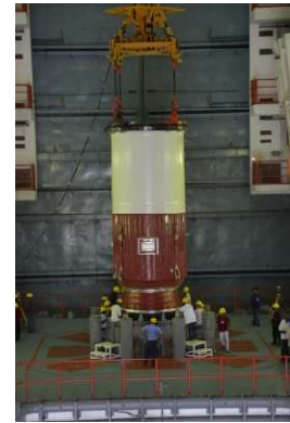
Placement of Nozzle end segment of GSLV-F11 Core stage
