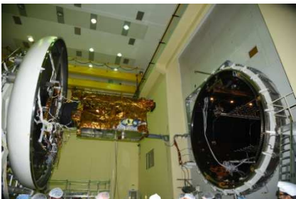
GSAT-7A being loaded into Thermovac chamber
