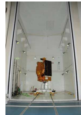
GSAT-7A undergoing Acoustic Test
